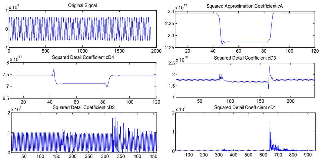
**Figure 5: Squared Wavelet Coefficient of Voltage Signal of Phase-a Using Db4 as Mother Wavelet with Sudden Connection of Load with Grid**
