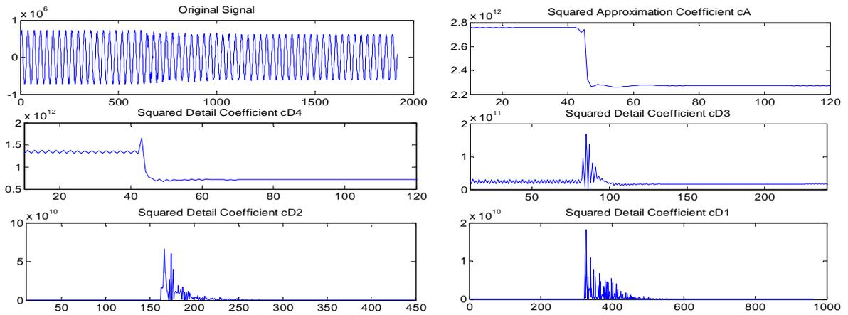
**Figure 7: Squared Wavelet Coefficient of Voltage Signal of Phase-a Using Db4 as Mother Wavelet with Synchronization of Test System with Utility Grid**
